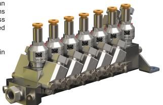
Each inlet block can be configured with or without recirculation, for pipes up to Ø8/10mm, with or without non-return valve. As an option, the pressure regulator type PT-REG can be directly integrated into the color changer. The whole system can then be used as a standalone unit or connected to the gear pump to offer a complete and compact system. This way you only have one technical partner for all the devices.
